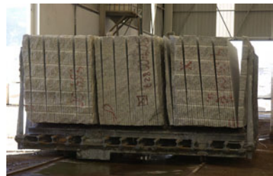
Quarry blocks fragmented in slabs
